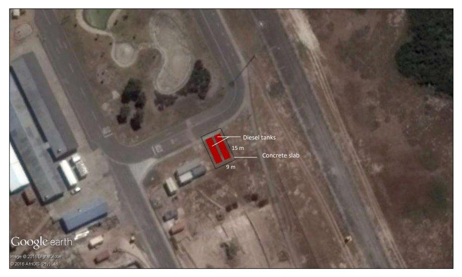
Figure 1: Illustration of the layout of the proposed diesel tanks at the Ekhaya site.
